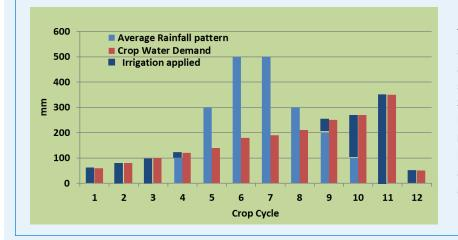
This graph describes typical sugarcane irrigation requirements for a crop cycle in dry winter and humid summer conditions. Several months of both complete irrigation and partial irrigation are required, while there is no need to irrigate during the peak rain season, although fertigation still must be applied in such circumstances.
