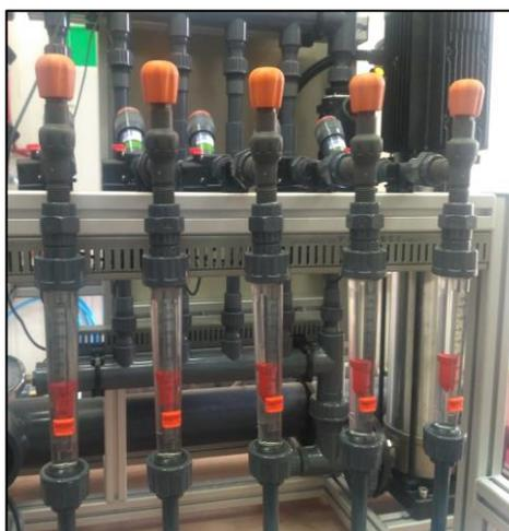
Example: If the observed rate is 100 liters per hour when set at 25%, the maximum rate should be 400 liters per hour (formula:  $100 / 0.25 = 400$ ).
