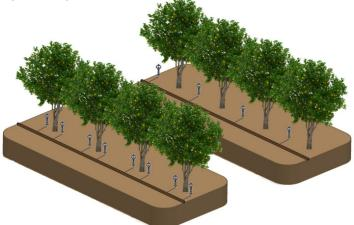
Plant spacing: 2-4m Row spacing: 5-7m Ridge spacing: 5-7m
