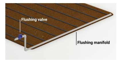
The flushing manifold is sized for a flow velocity of at least 0.5 m/sec at the end of the driplines to ensure sediment removal.
